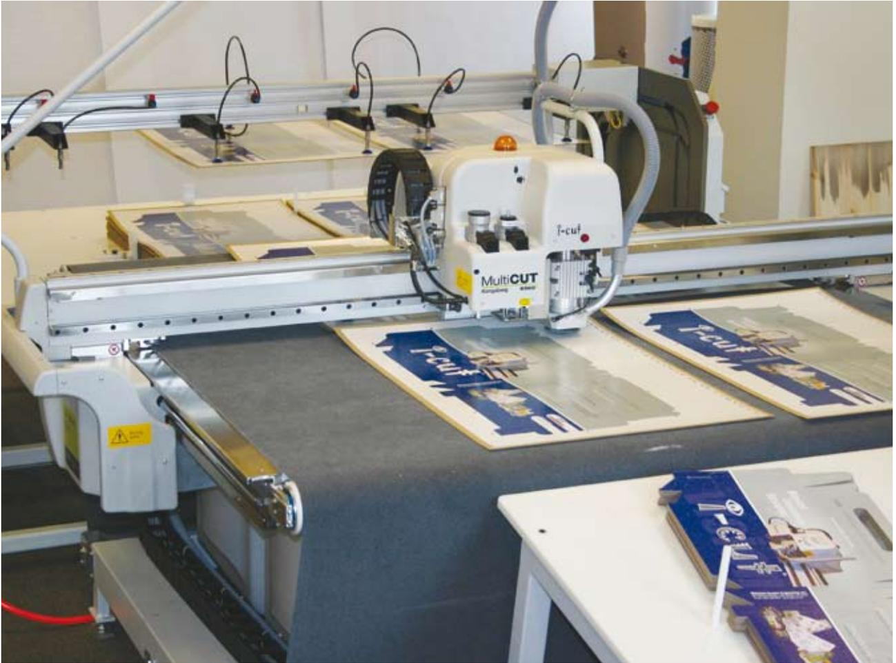
Material can be continuously retrieved from a roll of material, or sheets can be automatically fed through the MGE sheet feeding system.
